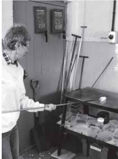
Janet rolls the glass through the dye to add the design colour.
